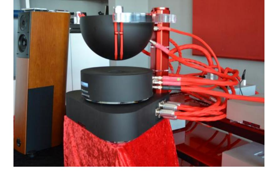
You can see the elastic system that suspends the chassis of the semispherical transport
